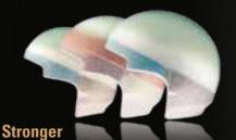
outer shell, softer inner shell Arai uses a stronger outer shell to spread impact forces and a softer inner shell to absorb remaining energy. The multiple-density EPS inner shell is made using a unique technology of combining three to five densities in various areas as a single component.
